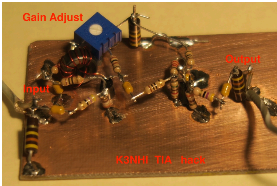
Fig 8. The amplifier that was measured in this note. The three half-watt 430K ohm resistors serve as mechanical supports and have nothing to do with the circuit operation.
