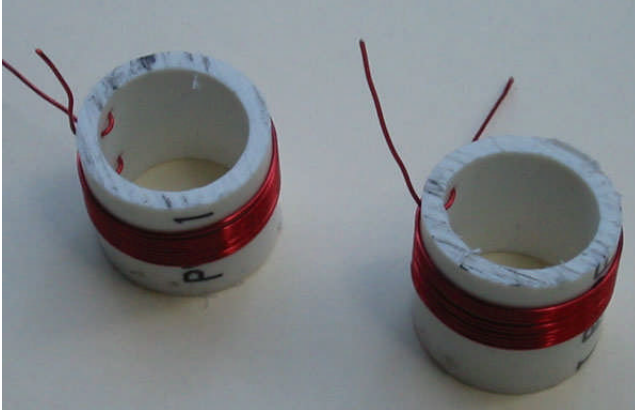
Coils wound on PVC Forms.
