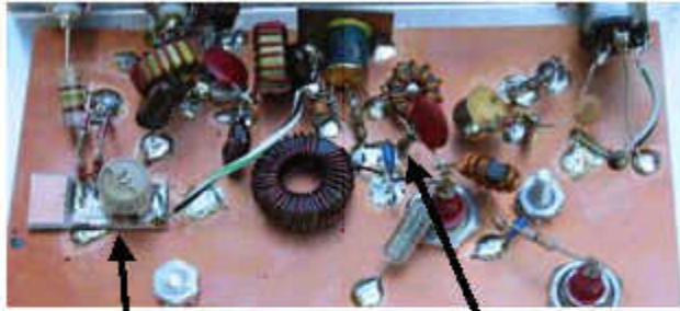
Added Support Resistor Trimmer Capacitor on PC Scrap, Glued to main Ground Foil. (Pre-Manhattan Period)
