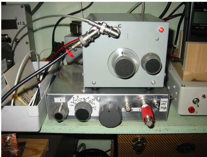
Fig 2. The upper gray box is an exterior view of the 8640-Jr. The lower box with three knobs is the RF source of fig 7.27, p 7.15 of Experimental Methods in RF Design (ARRL, 2003.)
