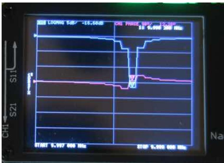
**Fig 22. Measurement of the Q of a crystal, 2 kHz total span.**
