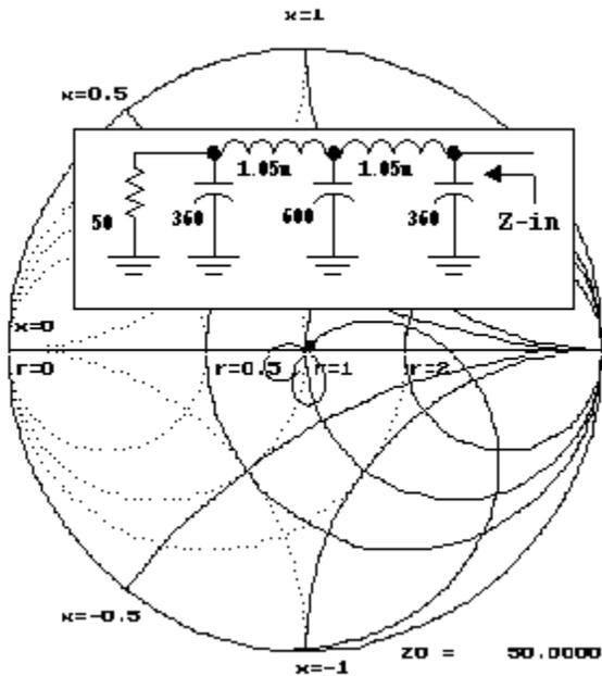
For an output of about half a watt with reasonable efficiency, we want the PA collector to see an impedance of about 100 Ohms with minimal reactance. We could insert a matching network or we can adjust the existing low pass filter to produce this value. The capacitor and inductor closest to the collector are adjusted until the 10.1 MHz impedance "seen" by the collector is close to the desired value, shown below.
