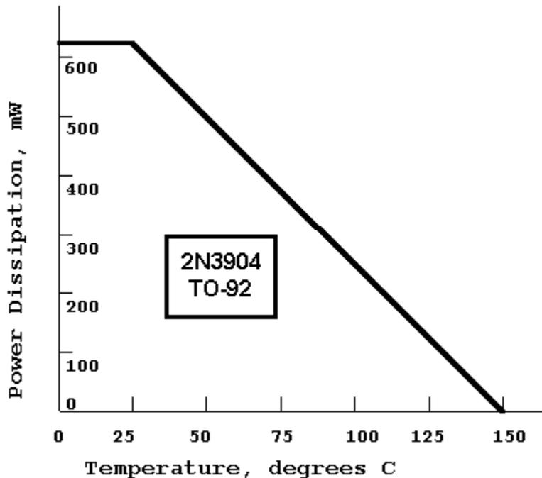
Other parameters are also significant, an important one being thermal resistance,  $R_{JA}$ . The 2N3904 has a thermal resistance,  $R_{JA}=200\text{ }^{\circ}\text{C/W}$  indicating a junction temperature rise of  $200\text{ }^{\circ}\text{C}$  for each watt dissipated in the transistor. The "JA" subscript indicates that this value describes the temperature difference between the junction and ambient, the surrounding air in this case.
