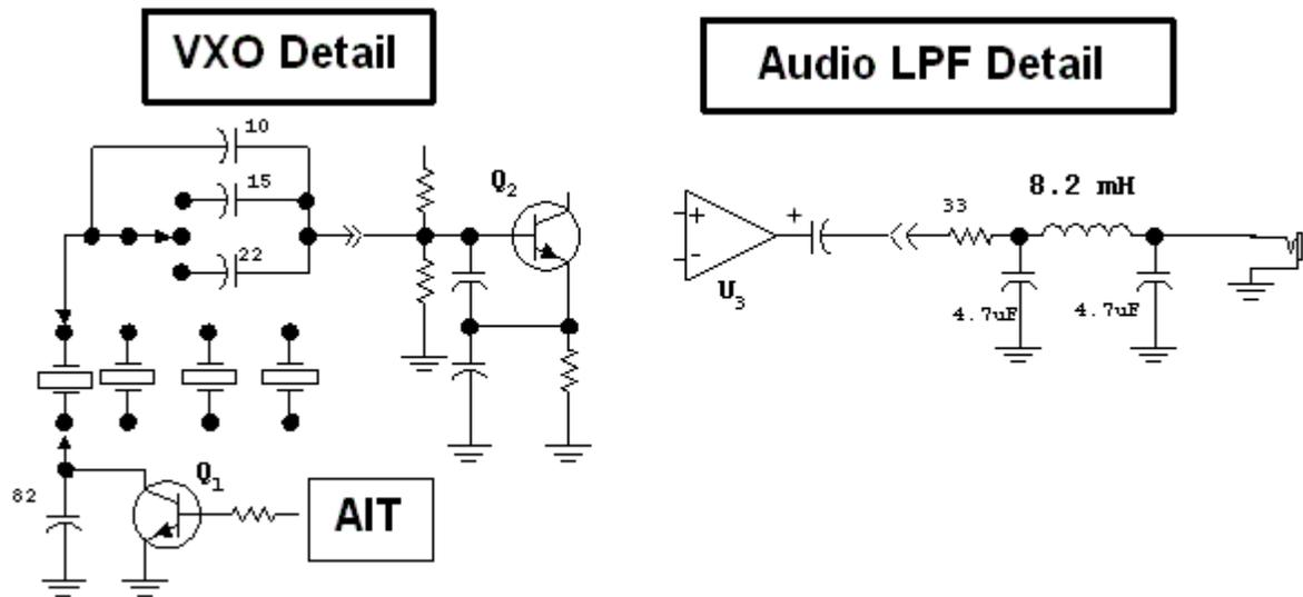
There is a lot of flexibility and room for experimentation here. The individual experimenter may need to change the VXO capacitors to hit the desired range. The audio filter is designed for a 1 kHz cutoff with a 35 Ohm source and load. But slight changes in L or C won't upset things badly, so use what you have available.
