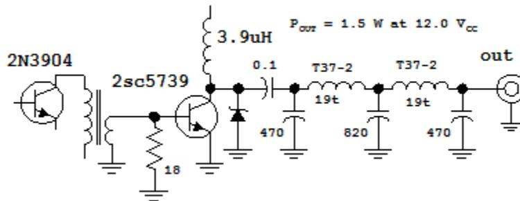
The RFC was replaced with one with a smaller inductance of 3.9 uH. The output network was redesigned to be a simple Chebyshev, then altered to an ultraspherical form to fit capacitors in the junk box.
