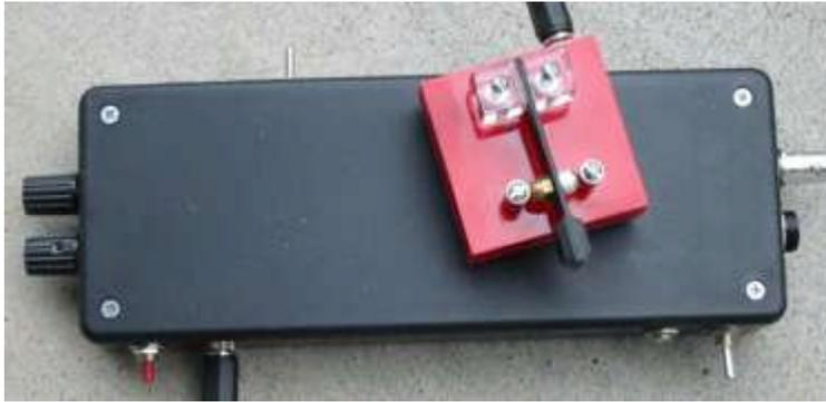
The transceiver is packaged in a 1 x 3 x 8 inch plastic box from Radio Shack, producing a transceiver weight of 8 Oz.
