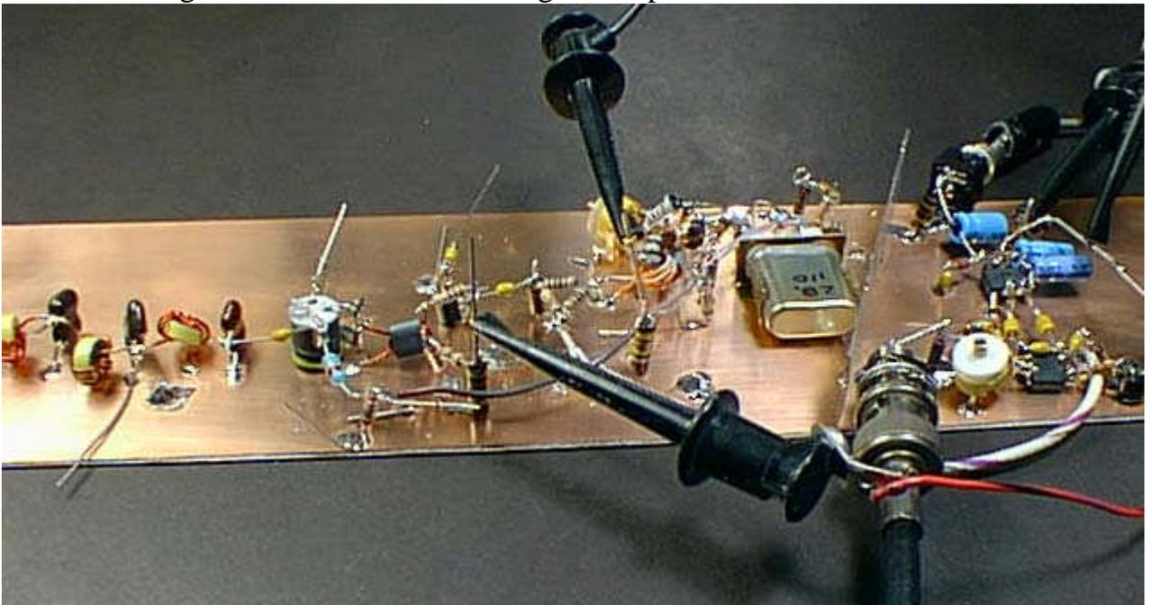
This version used a 2N3866 PA and had a 7th order low pass filter in the output. (Count the low pass filter components.) We switched parts later. We actually made contacts with this rig, even though it was less than convenient. But one could solder another strip to this one to form a "front panel" and have
