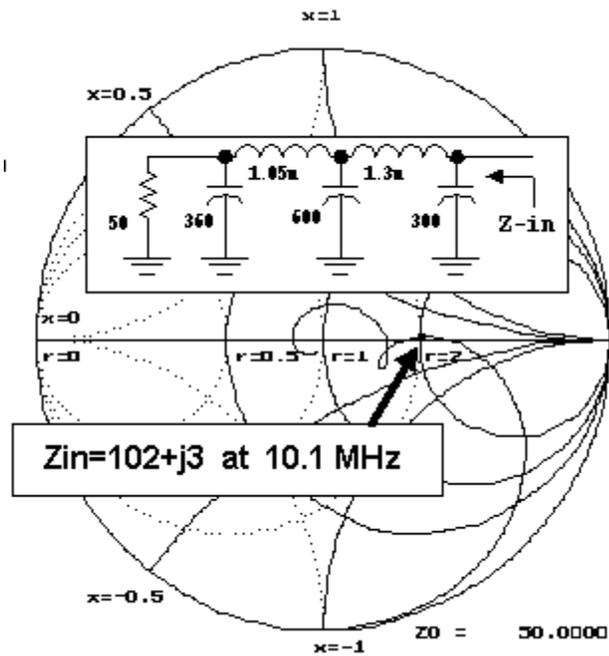
The final filter uses a 300 pF capacitor and a 1.3 uH inductor next to the collector. The reactance of these elements can be calculated at 10.1 MHz to generate a normalized filter that can now be used for any band, shown below.
