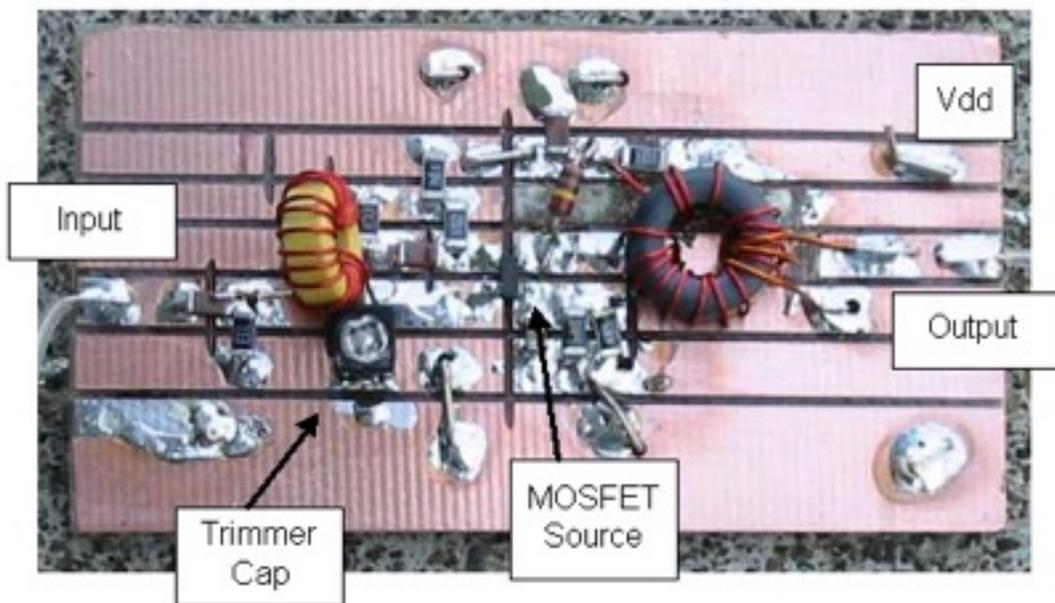
Note: The 1K lead in G2 was there mainly for layout convenience and could be eliminated. We used a 12 volt supply in our experiment, but the BF998 has a 12 volt drain-source breakdown. Hence, it would be better to use a lower Vdd, perhaps 6 or 8 volts. Gate-2 is biased at about 4 volts in our circuit. Changing the 100 K resistor with a new Vdd would preserve this bias. Experiment.
