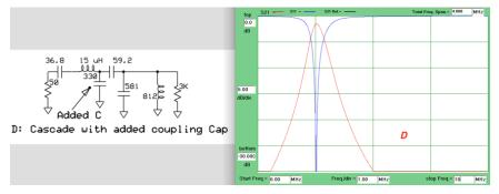
A recent transceiver ("**The Micromountaineer Revisited**," QST, July, 2000, pp28-33) suffers from this problem. It is solved at 7 MHz by adding a capacitor across J5. Any value from 330 to 470 pF should be fine. C12 and C20 will then need retweaking.
