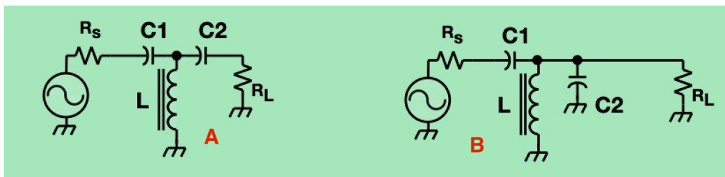
Fig 2. Two antenna tuner topologies. That at A works well with low and medium impedance levels while that at B works well for medium and high impedances.
