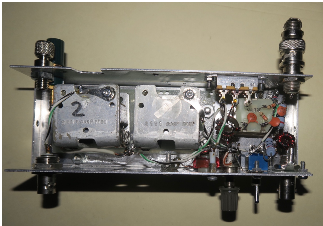
Fig 4. Inside view of the wide Z range transmatch. The isolated input is at the lower right along with the common mode choke. Binding posts are at the upper left while the low Z load port is at the lower left. The BNC connector at the upper right is not part of the circuit, but holds the male BNC that will short circuit the low Z output port when a high Z is to be matched.
