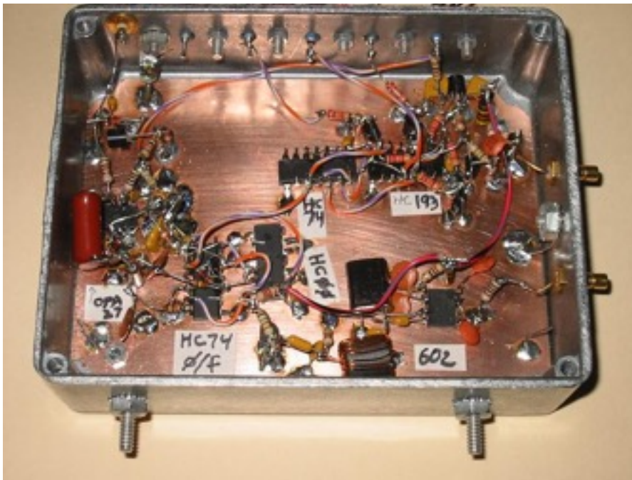
Fig 14. Interior view of synthesizer. The interface from the loop filter to the VCO is with coax.
