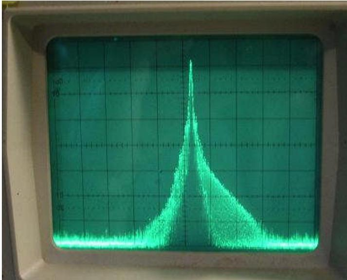
110 MHz 5<sup>th</sup> overtone crystal oscillator with squeezing. This signal was observed in a 12 kHz resolution bandwidth with a span of 0.5 MHz per division.
