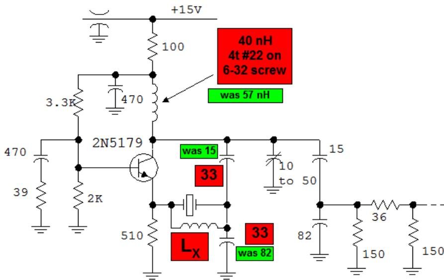
LX:  $-5 \text{ pF}$  at  $110 \text{ MHz} = 420 \text{ nH}$ , 10t #28 on T30-6
