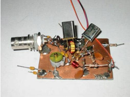
The modified crystal oscillator. This is the same oscillator board used to develop the original 1998 circuit. Many unused components, including a crystal, are tacked onto the board for later examination.
