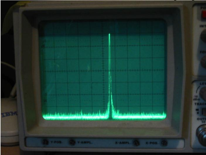
The output spectrum of the cleaner 110 MHz crystal controlled oscillator. The analyzer parameters are identical with the earlier photo.
